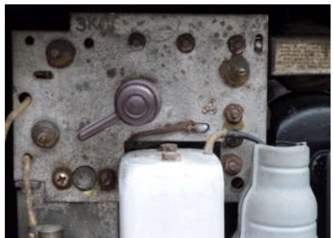
Shown above is the wave change switch on a 3K06.
